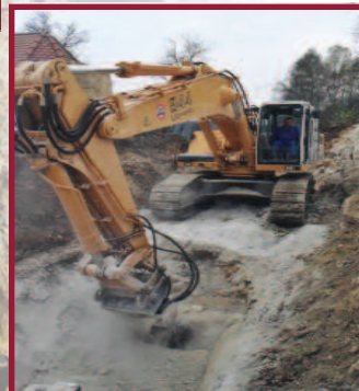
AQ-4 mounted on Liebherr 944 excavator working in medium hard limestone.
