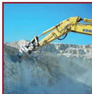
AQ-4 mounted on Komatsu PC400 mining Talc producing 100+ tons per hour
